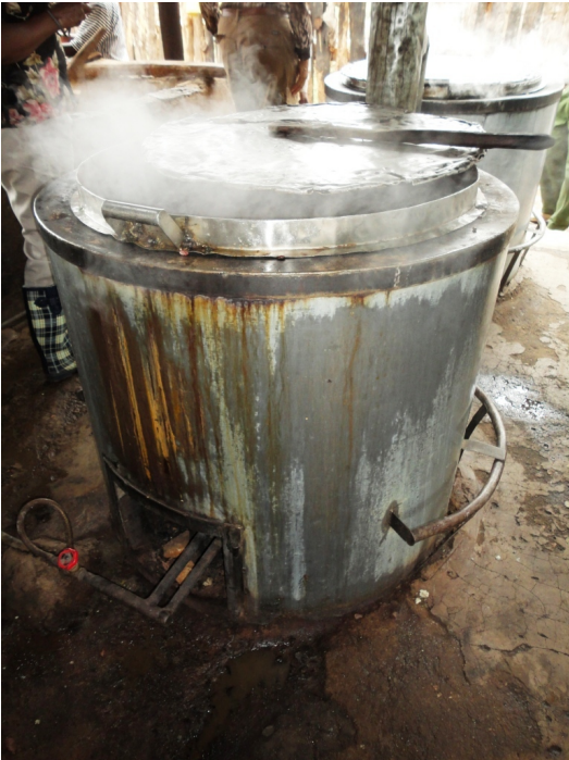
COOKING WITH BIOGAS FROM HUMAN WASTE IN THE PRISON USING LARGE IMPROVED STOVES
