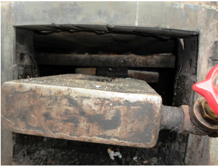
BIOGAS BURNER IN THE IMPROVED COOKSTOVE
