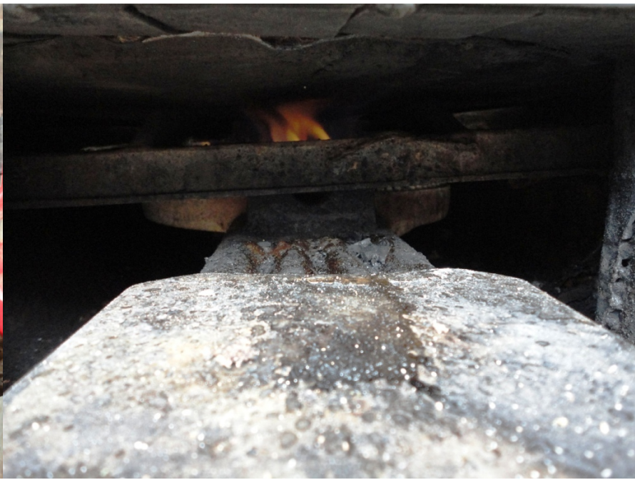
BIOGAS BURNER IN THE IMPROVED COOKSTOVE
